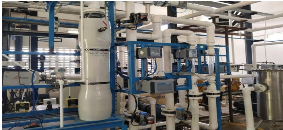
Fig B1: Picture showing 250 nm pilot scale ceramic membrane at STP, IITM.
